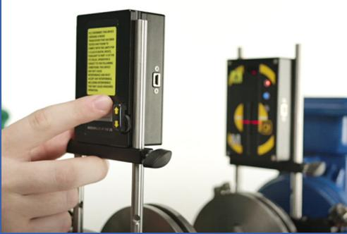
Adjust the position of the **measuring units** by moving them smoothly along the racks. After that, make sure that the measuring units are tightened securely on the rack.
