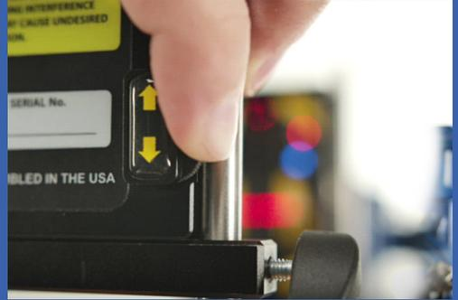
If the **laser beam** does not enter the center of the detector area, use the **adjustment screw** on the back housing to change the position of the laser beam to the centre of the **detector**.
