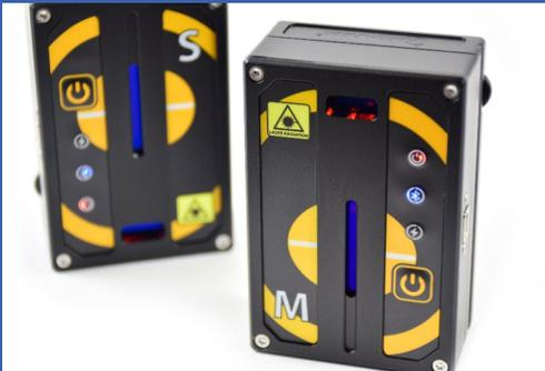
After the **measuring units** have been connected to the device, the **Bluetooth indicator** lights up **blue**.
