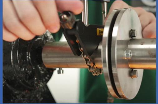
Tighten the **chain** with the **tightening screw**. Do not use excessive force.
