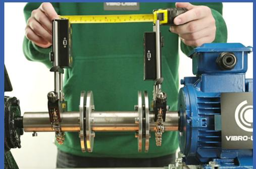
It is recommended, in order to achieve the highest measurement accuracy, to install the **measuring units** so that the distance between them is as large as possible, ranging from **0.1** to **10 m**.
