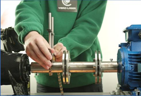
Hold the mount with the **draw chain** vertically and install it on the shaft. Raise the free end of the chain, stretch it, removing the slack, and fasten it on the clevis.
