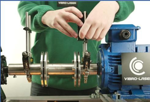
Place the measuring **units M** and **S** between the racks so that the screw bar is under the measuring units.
